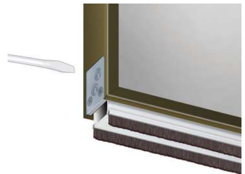
Adjust Bottom Brush at hinge stile
