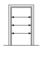
Measure height at each side of opening, a few inches in from the jambs and in the center. Record the shorter dimension.
