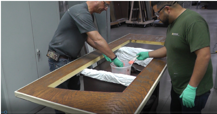
Mask off the aluminum perimeter
