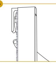
Square mullion to floor (side to side). Mark bracket position. Screw on bracket.
