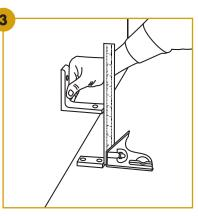
Locate block on floor using bracket against wall. Mark block position. Screw down block.
