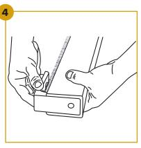
Position top bracket on rod to check fit.
