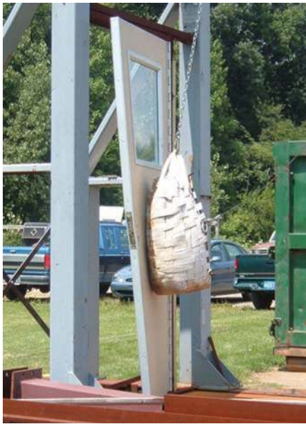
This lightweight, flexible FRP door was tested for structural strength by repeatedly slamming it with a bag filled with 215 pounds of sand. The distance was increased incrementally until it reached a force of 750 ft-lb.
