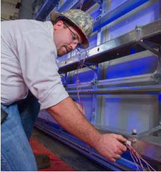
Strain gauges being installed on subject door prior to testing.
