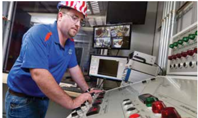
J. Alex Esposito, M.E., E.I.T., lab manager, Powell Family Structures and Material Lab at the simulator’s analog control panel designed by Henry Upjohn. Monitors and equipment for digital test data capture are seen in background.
