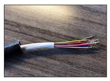
It is possible to run up to 12 wires through Special-Lite conduit with the Molex pin & socket crimps installed.
