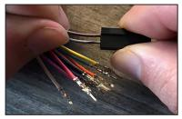
Once it is in all the way you won't be able to see the crimped on pin connector. Gently pull on the wire to ensure that the pin connector is locked in place inside the plastic Molex connector.
