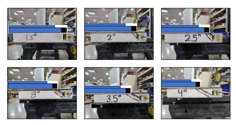
On the hinge stile of the door, there is a 3/8" x  $\frac{3}{4}$ " channel that runs the length of the door located 1.5" off of the edge, pictured above. In order to access this channel:
