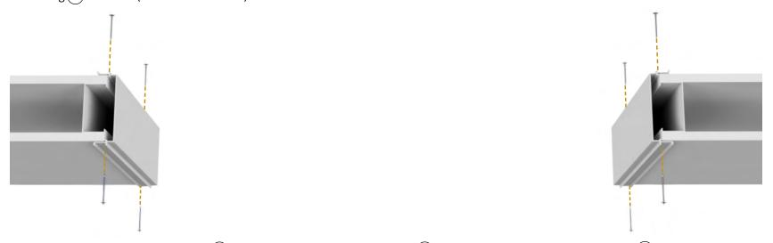
B. Anchor Jambs using fasteners: Bag (B) Metal Stud (SL-SCP-SDLH200), Bag (D) Wood Stud (SL-SCP-FTLH200), or Bag (I) Concrete (SL-SCP-THW14214). Place fasteners 3" from each end and no more than 16" apart (both sides should roughly align).
