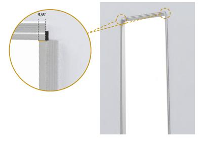
C. When vertical jambs are set and square, the header should overlap the jambs by 5/8".
