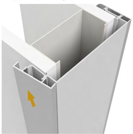
A. Snap on the trim by hooking the outside leg on first, then tap lightly with a mallet (optionally add wood block) toward the inside to snap on. One square-cut piece of trim should remain (to be used in the next step).
