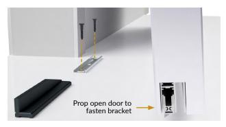
C. Install the Floor Guide Bracket using the included fasteners, and then slide the Drop Seal Floor Guide into the door bottom channel again, sliding it into place in the bracket until you hear it click. Test the door to ensure the Drop Seal functions correctly and adjust as needed.
