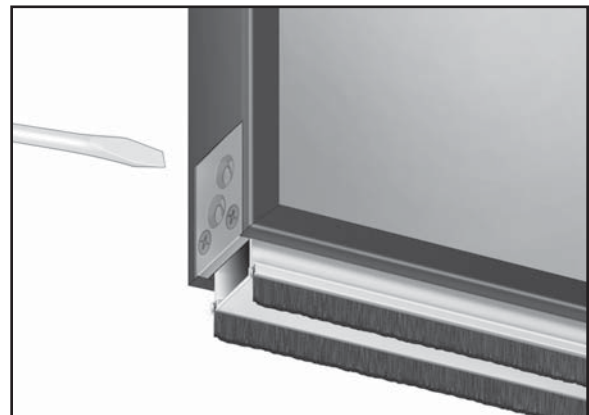
Adjustment of bottom brush on hinge side of door
